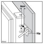
9. Remove the squares and mark a distance of 8 mm from the outer edge of the door where the nail must be fitted (K).
